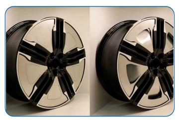
reduce air resistance in the single-digit percentage range. More would be possible, but only closing the rim completely could more effectively stop the flow of air and the damaging rotor effect of the wheel. This, in turn, is in direct conflict with the necessary cooling of the brake chamber, especially in cases of higher loads, for example when descending
