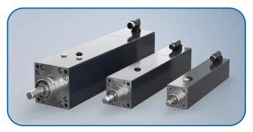
At the end of the shaft of the spindle is an external thread, on which commercially available adapters such as e.B. Ball heads or clamping hooks from the pneumatic/hydraulic range can be mounted. The flange dimension of the electric cylinder is based on ISO 15552 and has screw-on points on both sides if an application requires e.B a swivel eye connection. This compatibility makes the switch from pneumatics to electric drive technology particularly easy.
