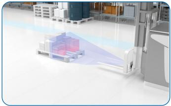
It includes two device variants with their own measurement methods on one platform: Stereo Vision and Timeof-Flight. Housed in the same housing, with uniform user software and data output, the integration effort for 3D applications can be significantly reduced.
