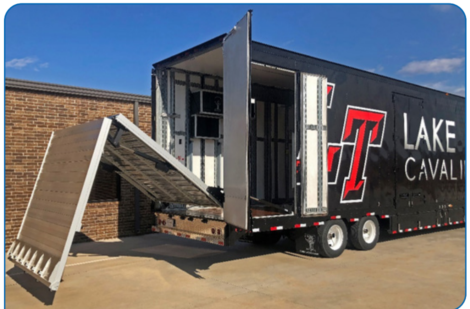
Figure 3 The synchronization feature of the Thomson Electrak HD helps coordinate smooth, safe and quick ramp operation.
