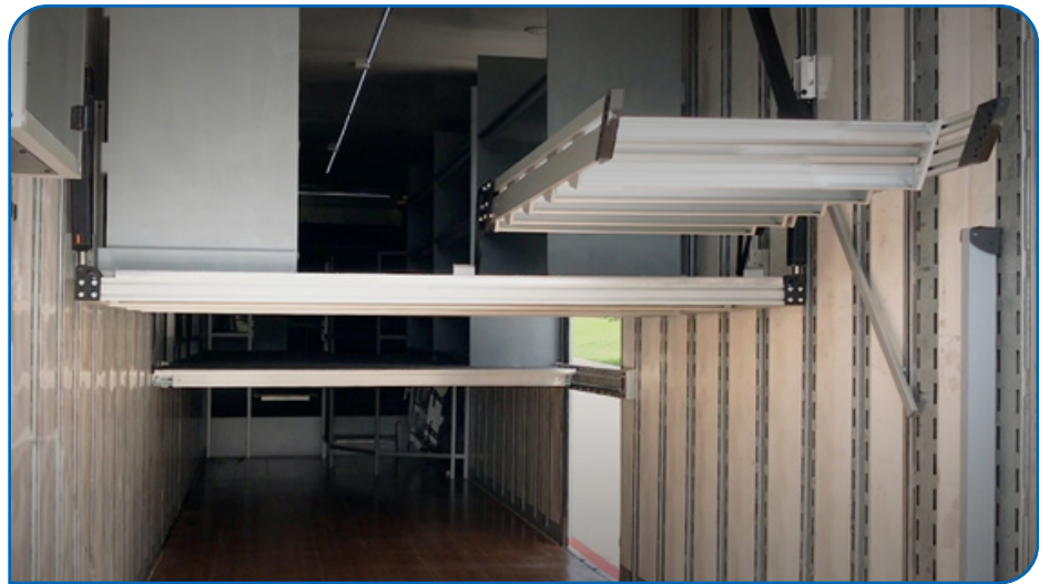
Figure 4 Actuator synchronization enables operators to raise this moving floor up to increase storage space.
