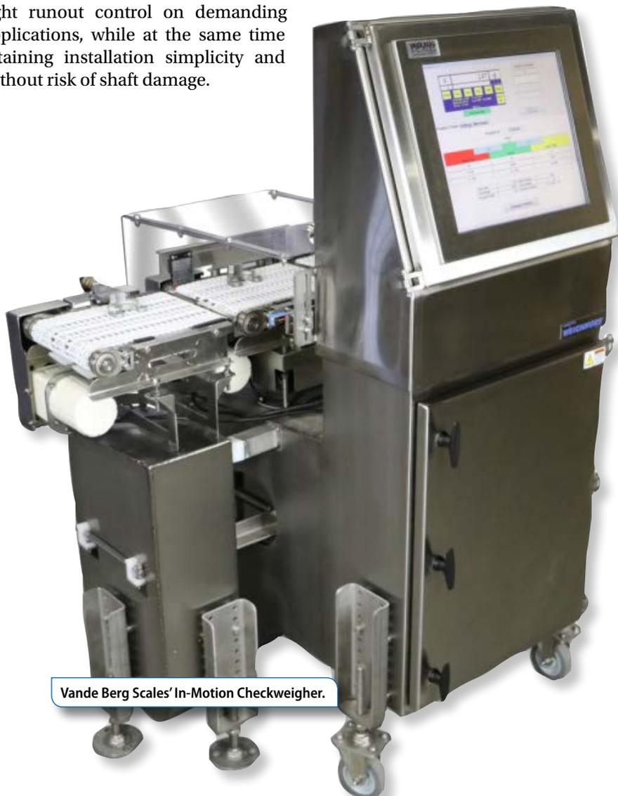
Vande Berg Scales' In-Motion Checkweigher.
