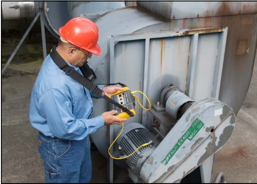
Figure 5 Technician using a handheld vibration analyzer.
