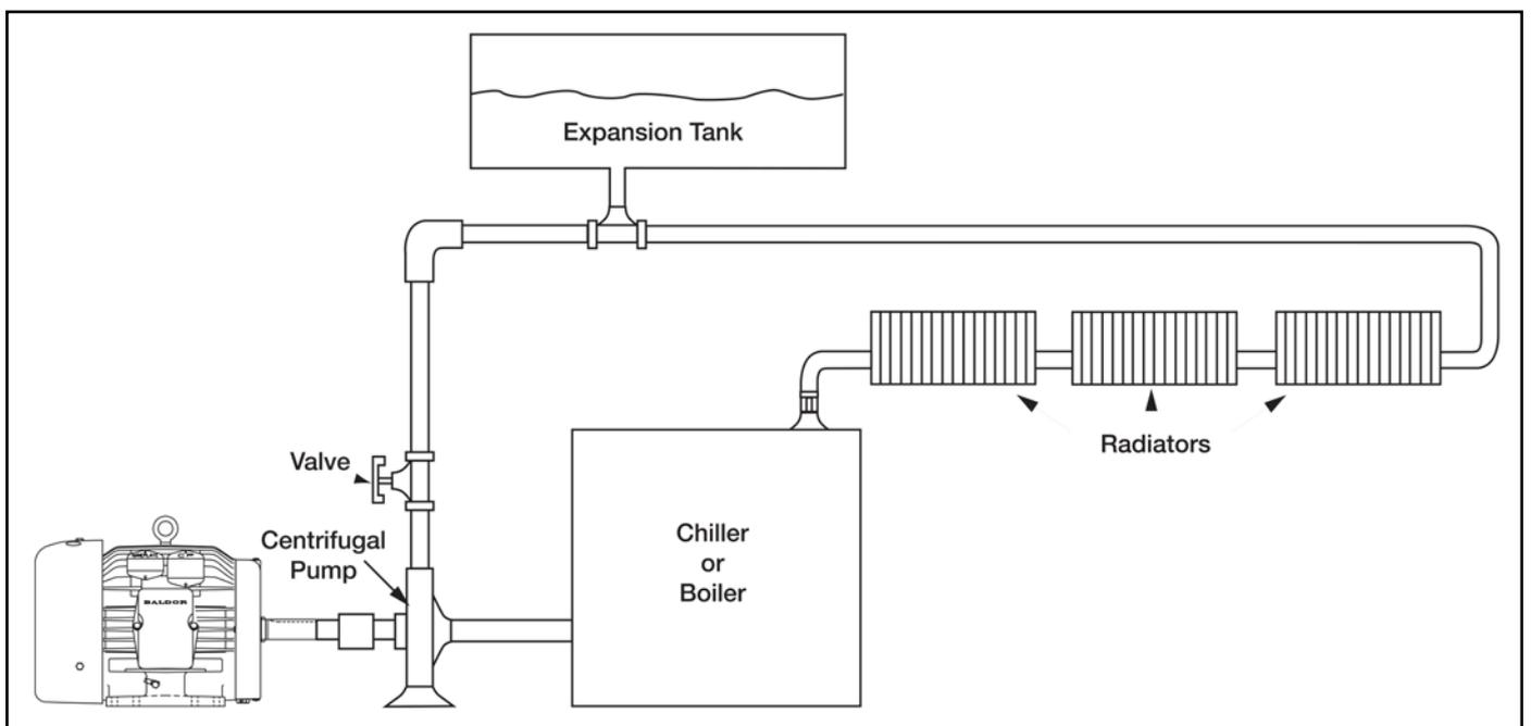
Figure 1 Pump arrangement circulating chilled or hot water through a closed system.
