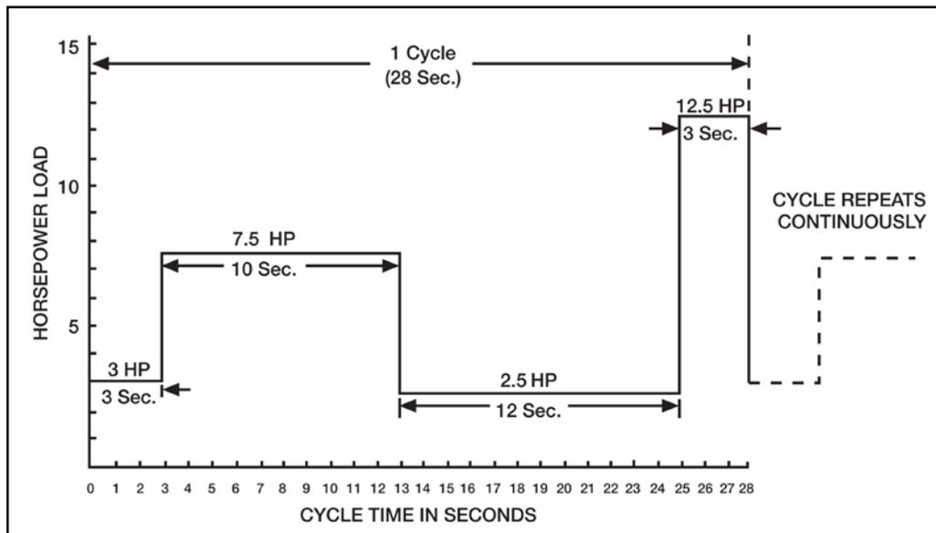
Figure 1 Using RMS method of horsepower determination requires that duty cycle is spelled out in detail (Fig. 1).
