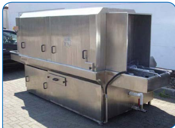
Corrosion resistant bearings should be considered for the live bird crate washer.
