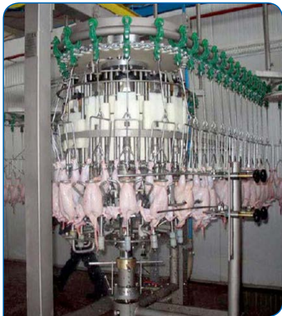
The use of stainless steel radial ball bearings ranging in sizes from 6201 to 6205 can be utilized for the vent remover in the poultry process.
