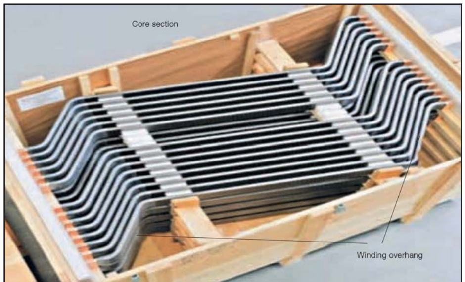
Figure 6 Full vacuum pressure impregnation for windings.
