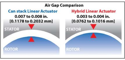
the can stack motor, resulting in the hybrid motor's higher efficiency. series, i.e. — 1.8 degree/step and .9 degree/step (vs. 7.5 or 15 degrees for the typical can stack) will allow resolutions down to .000060 in. [0.001524 mm]/full step compared to .00025 in.[0.00635 mm]/full step in a can stack motor. Therefore the hybrid motor provides much finer positioning capability.
