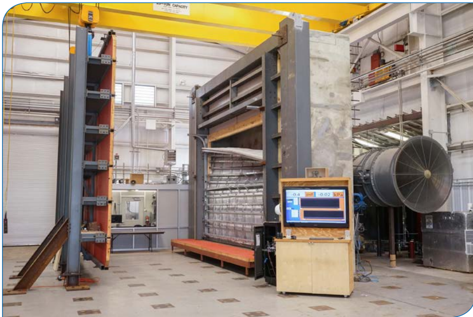
Damaged sectional roll up door following test (all photos courtesy of Altra).
