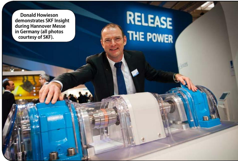
avoid many health problems before they occur. In a similar way, SKF Insight enables you to monitor the bearings' operating conditions, understand the complex history of load in service and quality of lubrication throughout life. It can also identify overloads, duty excursions, lubricant contamination and lubrication problems so that modifications can be made to the operating conditions to avoid damage before it occurs."
