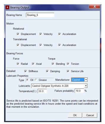
Figure 5 Bearing output window.
