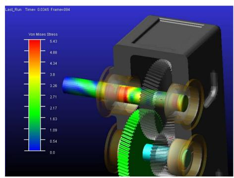
Figure 3 Stress distribution of the input shaft.
