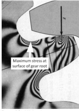
Figure 1 Failure initiation points.
