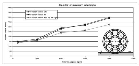
Friction torque at minimum lubrication.
