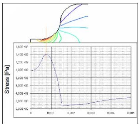
Figure 9 FEM calculation of highest-stressed region.
