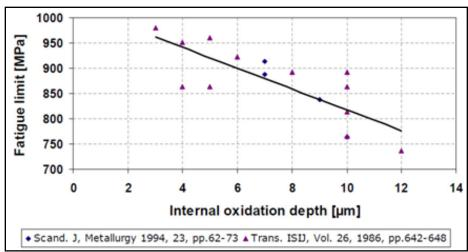
Internal oxidation and fatigue limit: literature indicated a potential gain of 100 MPa in the fatigue limit if the internal oxidation is restricted to 2  $\mu$ m maximum.
