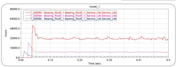
Figure 6 Bearing service life under different input torques.
