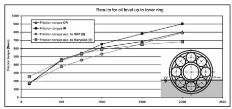
Figure 4 Friction torque at oil level "up to inner ring."
