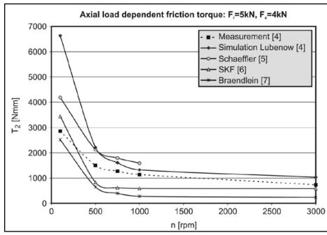
Axial load-dependent friction torque  $T_2$  according to different calculation methods and measurement results.
