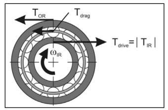
Figure 2 Measured friction torques of a bearing.
