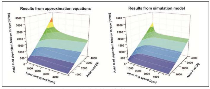
Figure 9 Results from the approximation equations vs. results from the simulation model (Ref. 9).
