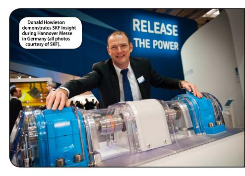
avoid many health problems before they occur. In a similar way, SKF Insight enables you to monitor the bearings' operating conditions, understand the complex history of load in service and quality of lubrication throughout life. It can also identify overloads, duty excursions, lubricant contamination and lubrication problems so that modifications can be made to the operating conditions to avoid damage before it occurs."
