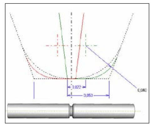
Figure 8 Notched test sample and gear root geometry.
