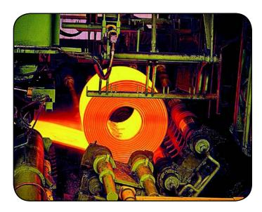
Motors driving rollers are subjected to sudden torque variations, sometimes from zero to overload, immense acceleration requirements and frequent rotation reversals. WEG has designed its motors with high starting and breakdown torques so that they operate exceptionally in these conditions. Depending on the application, WEG can also customize the right solution to fit the individual need.
