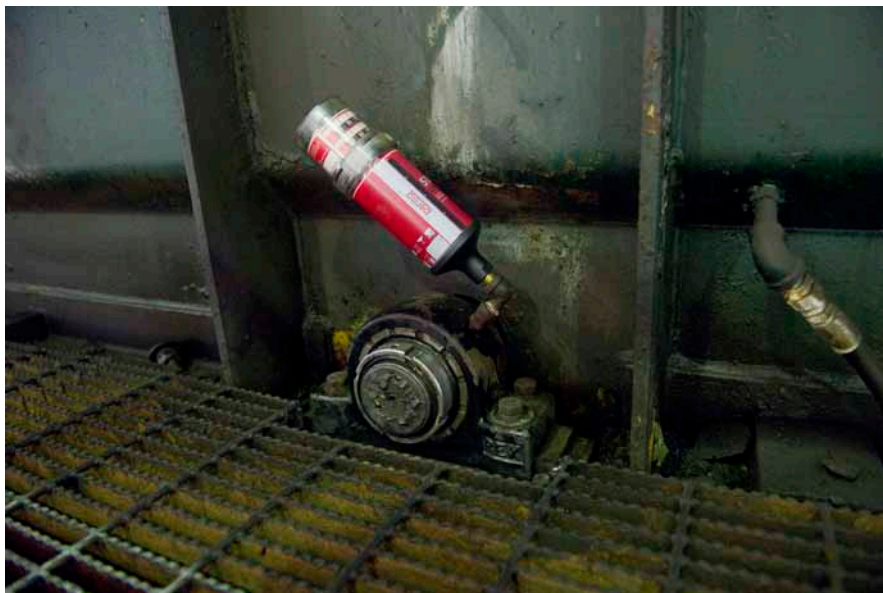
Bearings operate in a difficult environment on this quench tank application. Impact of tubes entering tank caused the roller shaft to move sideways with previous bearings.
