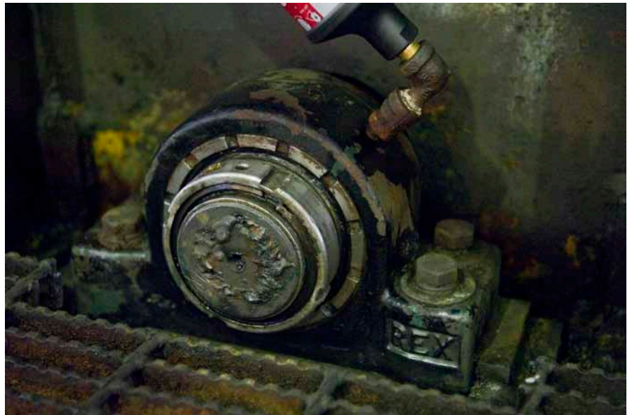
Rexnord ZA6215F adapter mount roller bearings with Shurlok technology incorporate a tapered locking sleeve to maintain bearing position on this quench tank.
