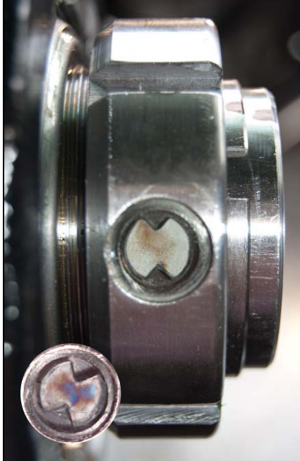
Optical Strain Sensing (OSS) technology in new bearings changes color to tell the installer when the bearings have been correctly tightened to the shaft.
