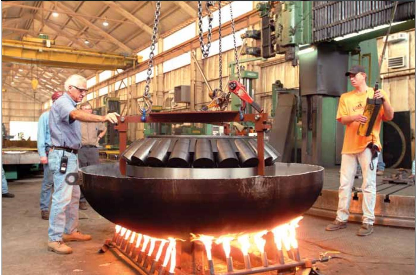
The final mounting and horizontal preheat of a large bearing for a New York bridge application (courtesy of SKF).
