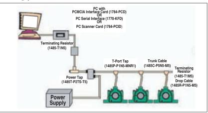
Figure 3—Condition monitoring system set-up (courtesy of Baldor-Dodge-Reliance).
