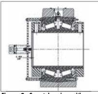
Figure 2—Smart bearing with speed proximity switch (courtesy of Baldor-Dodge-Reliance).
