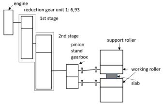
Figure 2—Drivetrain of a rolling mill.
