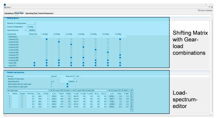
Figure 1—Shifting matrix with gear-loaded combinations and load collective editor.
