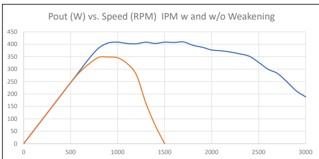
Figure 9—Output Power vs. Speed for Indirect PMSM with and without field weakening at 100% torque.
