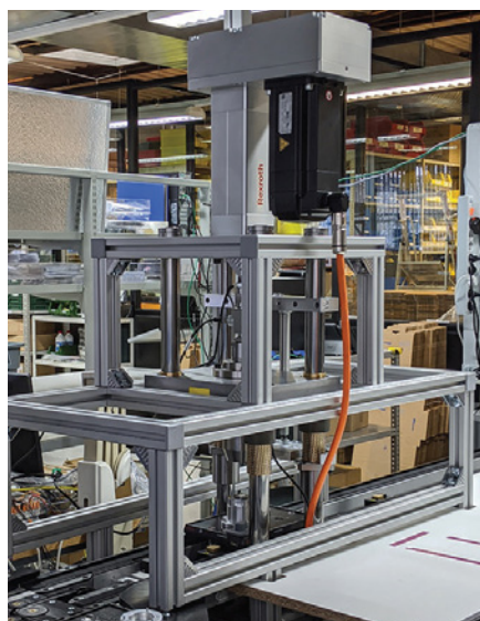
Production of different types of rotary encoders at Sensata: the Smart Function Kit for Pressing reduces engineering, commissioning and quality assurance costs. (Copyright: Sensata)
