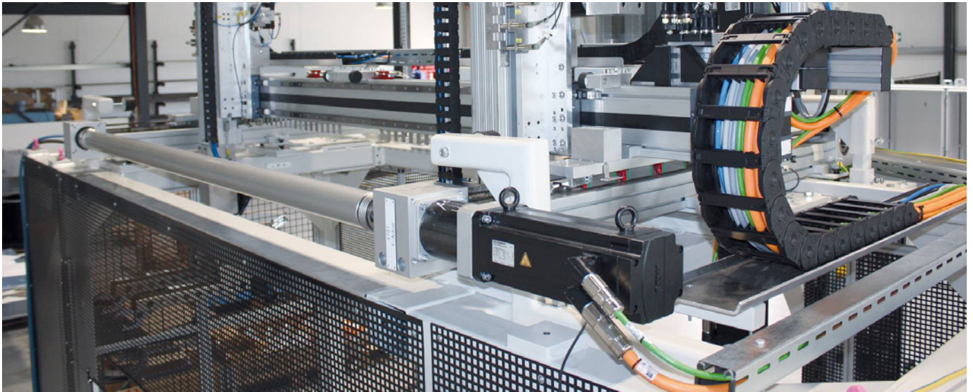
Torsionally stiff line shaft couplings are ideal for linking belt-driven linear actuators which will be used in tandem to support the loads overhead.
