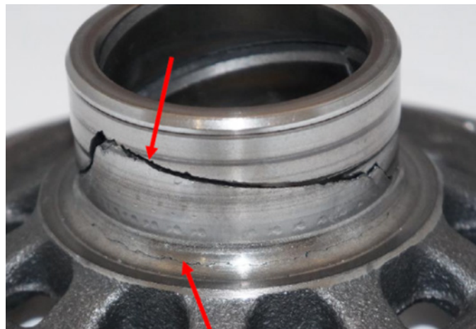
Figure 1 — Differential hub cracking on high load test due to wear of material from insufficient press fit.
