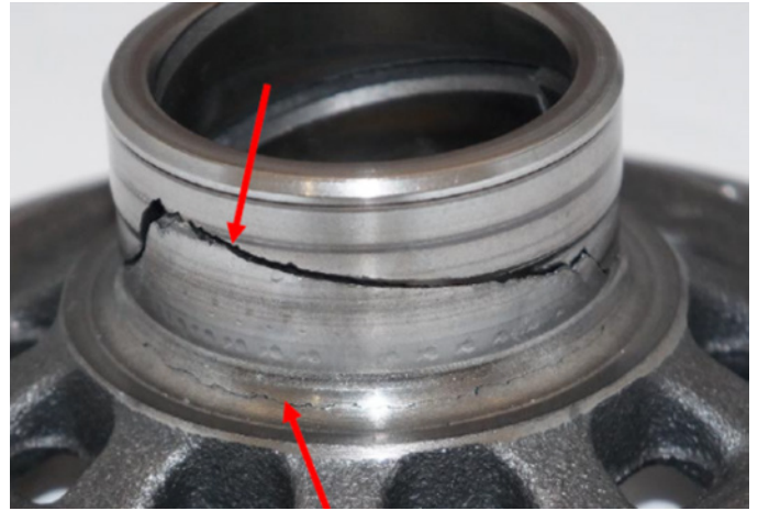
Figure 1 — Differential hub cracking on high load test due to wear of material from insufficient press fit.
