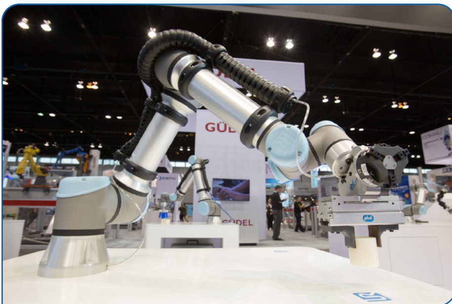
The PHD series offers seamless integration for Universal Robots that utilize standard PHD pneumatic grippers.
