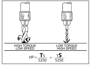
Figure 4 Constant HP Speed-Torque Relationships
