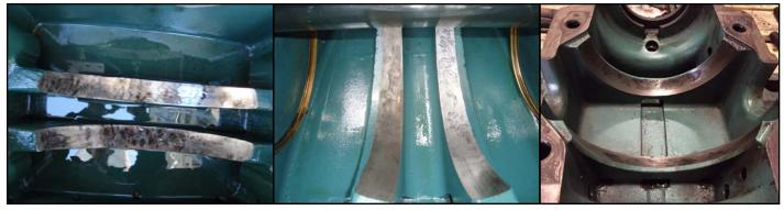
Figure 4 Three separate housings that have been pulled from service due to high fan vibration levels and exhibit the characteristic fretting marks caused by improper contact and retention of the liner within the housing.
