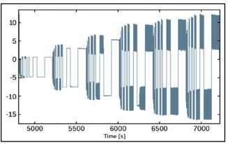
Figure 8 A stick-slip curve of BR non-standard bearing material at 1° angle.
