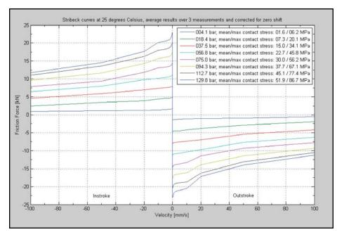
Figure 3 A Stribeck curve of supplier sample bearing material at 0° angle, general results at 25°C.
