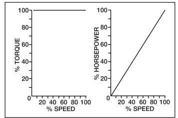
Figure 3 Constant Torque Speed-Torque Relationship
