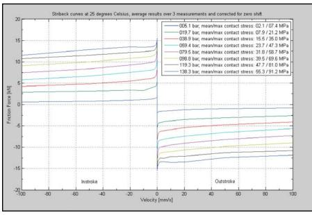
Figure 5 A Stribeck curve of LHC manufacturer standard bearing material at 0° angle, general results at 25°C.
