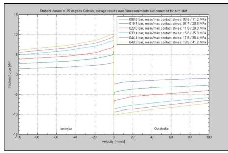
Figure 4 A Stribeck curve of supplier sample bearing material at 1° angle, general results at 25°C.
