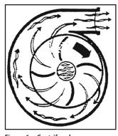
Figure 6 Centrifugal pump — variable torque load.
