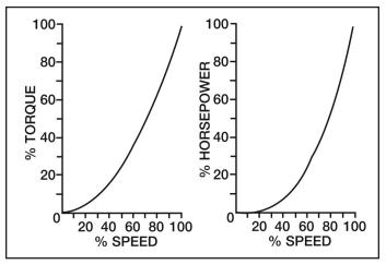
Figure 7 Variable torque — speed-torque relationships.
