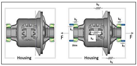
Figure 2 Where and how differential is fixtured.
