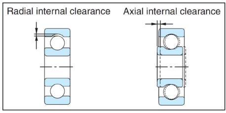
Figure 1 Distinguishing bearing radial internal clearance from preload tapered bearings (axial preload/endplay).
