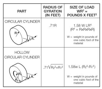
Figure 8 Formulas for determining radius of gyration and *WR*<sup>2</sup> of two frequently occurring cylindrical shapes: wt.: steel = 490; cast iron = 450; aluminum = 165.
