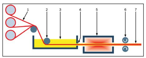
Figure 2 The key steps in the pultrusion process include: 1) continuous roll feed of reinforced fibers/ woven fiber mat; 2) tension control roll; 3) resin impregnator bath; 4) resin-soaked fiber; 5) bearing die and heat source; and 6) fiber pull mechanism.
