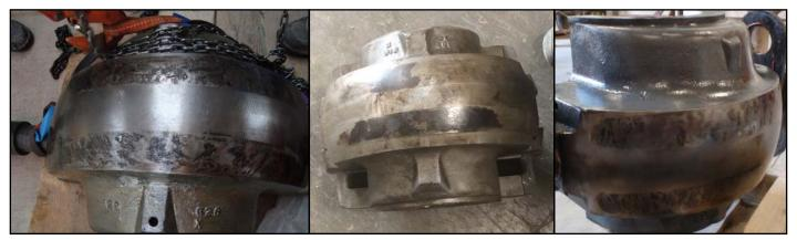
Figure 3 Three separate liners that have failed due to high fan vibration levels and show the fretting corrosion marks along their spherical seats.
