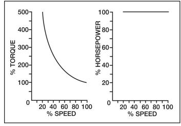
Figure 5 Constant HP speed /torque relationships.
