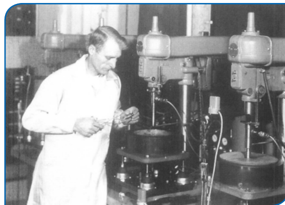
Eldred Johnson, chief technician for bearing research at NASA Lewis, with NASA five-ball fatigue testers on January 20, 1960. The fatigue tester was conceived by William Anderson, designed by Thomas Carter and Erwin Zaretsky, and assembled and operated by Johnson. The first tester began operation in March 1959. Eight testers were built by NASA. Over one-half-million test hours had been accumulated and reported before NASA terminated the research in October 1964. (All historical photos courtesy STLE.)
