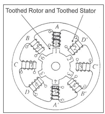
Figure 1 A detail showing six rotor teeth and eight stator teeth of a step motor, which uses a magnetic attraction process when the windings are energized sequentially — A, B, C, D — in a simple, counterclockwise direction.
