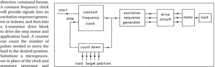
Figure 5 Driving and controlling an open-loop-configuration step motor provides the user with a simple pulse and direction command format.
