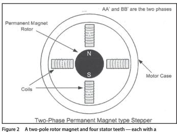
Figure 2 A two-pole rotor magnet and four stator teeth — each with a copper winding and an operating excitation sequence of A, B, A1, B1. There are some military and space applications that use this motor type with a rare earth rotor magnet.
