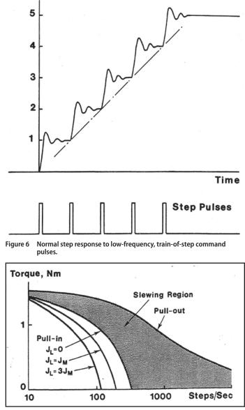
Figure 7 A typical curve for a hybrid step motor. There are two major elements in a step motor performance curve: the pull in, and pull out, torque regions.
