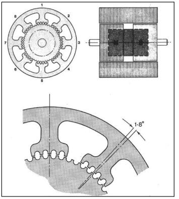
Figure 4 A hybrid (200 step/rev) stepping motor. The detail shows the rotor and stator tooth alignments, and indicates the step angle of 1.8°.
