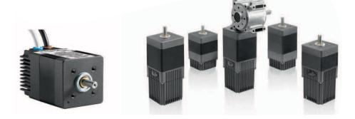
and 150 watts nominal usable power at 24VDC and support 9-56 VDC. The SMi21 incorporates a quality 4096 step encoder that controls position, torque, speed, direction, braking and other functions and includes 6 inputs and 4 outputs. Suitable uses include a variety of access control applications such as automatic doors and screen doors used in metro systems, trams, trains, and bank airlocks; as well as turnstiles, barriers and motorized traffic controls.
