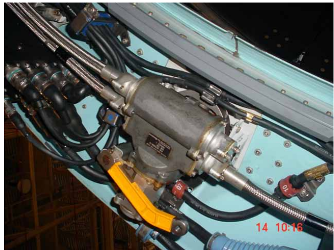
This is the center of an actuator which feeds power to the two adjacent actuators. So one shaft comes in and powers the center actuator and two shafts leave to power the adjacent actuators.
