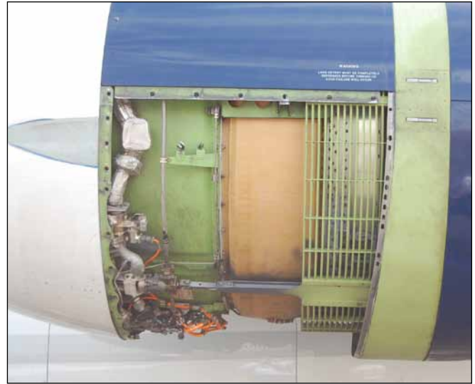
The Bombardier RJ200 plane with GERJ34 engines. The flexible shaft is visible going into one of the actuators which make up the Thrust Reverser Actuation System (TRAS).
