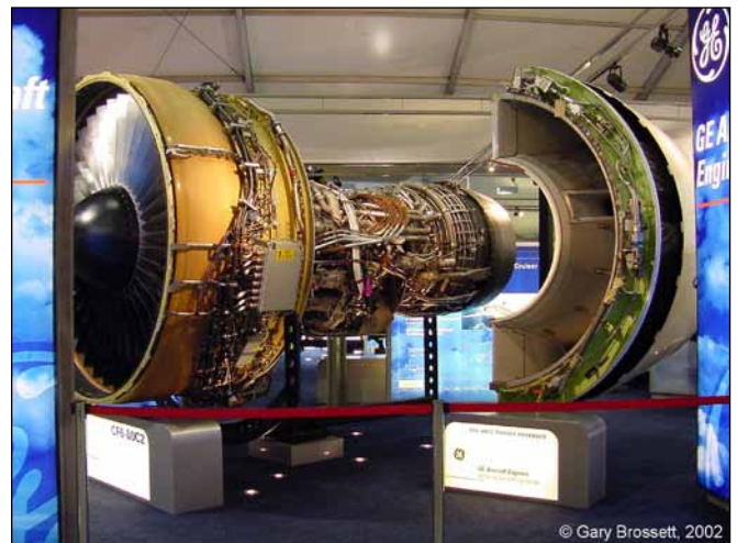
The right hand side of this photo shows the flexible shafts ringing the nacelle and attaching to the actuators.
