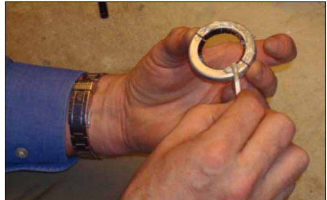
Figure 3—Narrow band of Aegis colloidal silver coating is then applied around the shaft to improve surface conductivity. Ring is then installed on the shaft and re-taped.
