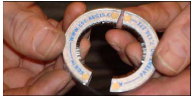
Figure 2—Equal proportions of epoxy and activator are mixed and small amounts are applied to the back of the ring.
