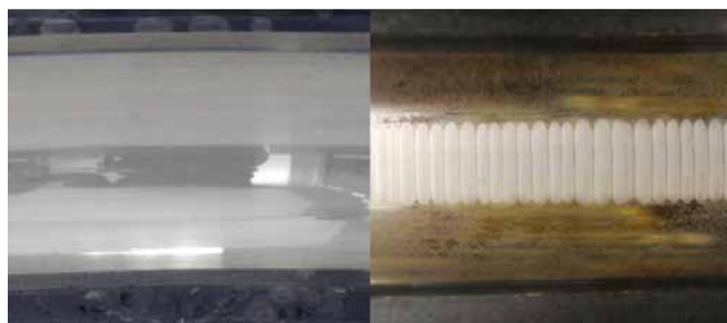
Figure 8—New bearing (left); fluted bearing (right).
