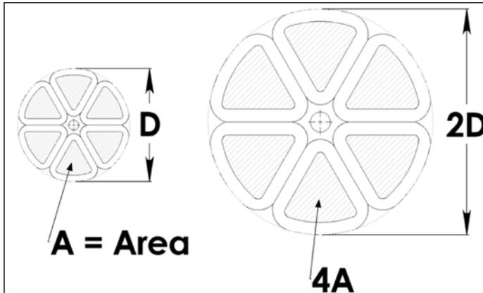
Figure 6—Axial motor with diameter  $D$  and  $2D$ .
