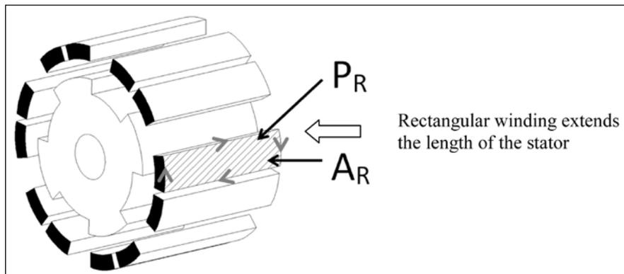
Figure 1B—Radial motor winding.
