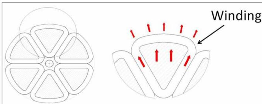
Figure 8—Axial motor thermal path.
