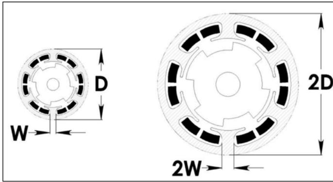
Figure 5—Radial motor with diameter  $D$  and  $2D$ .
