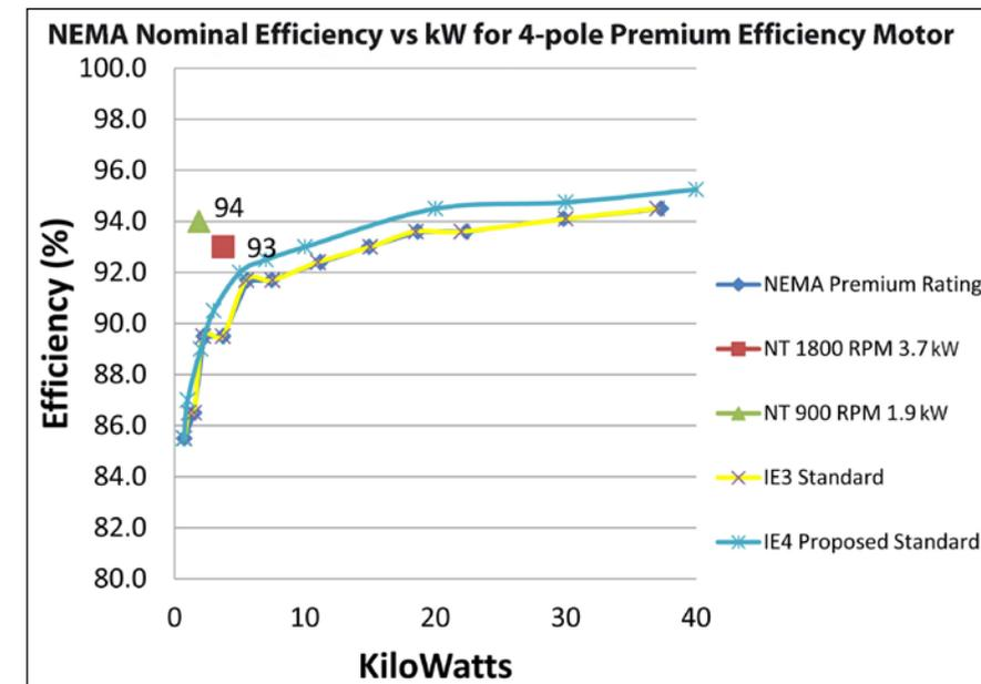
Figure 12—NEMA Premium Efficiency, IE3 standards and predicted motor efficiency.
