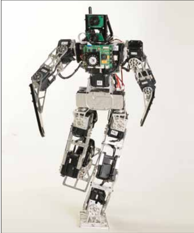
DARwin, a humanoid robot developed by the Robotics and Mechanisms Laboratory at the Virginia Tech University, is driven by motion control products from Maxon Precision Motors (courtesy of Maxon).
