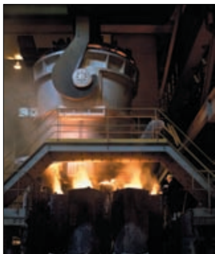
The bottom-pour operation processes steel at Timken’s Faircrest Steel Plant (courtesy of Timken).
