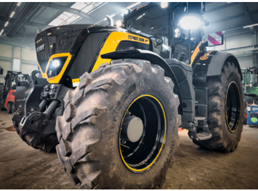
A Bluetooth enabled sensor inside Continental's tires gives farmers easy access to essential tire data directly on their mobile devices.
