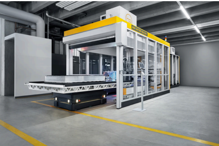
HAHN Automation Group has developed a battery tester that carries out a complete test of the mobile energy storage units fully automatically.
