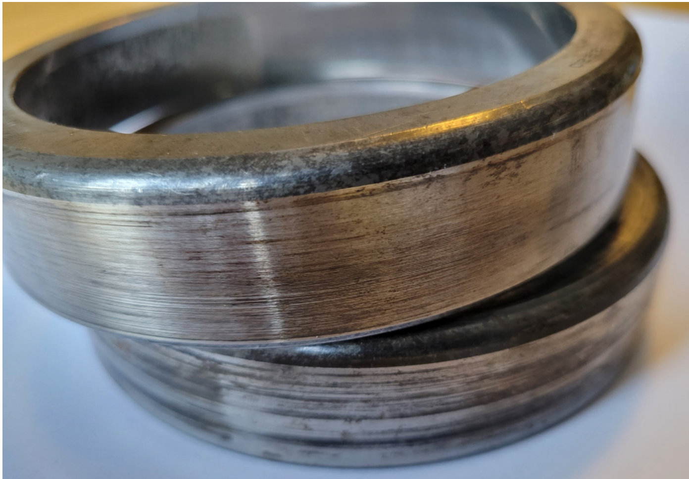
Figure 1—Outer ring creep of differential tapered bearings.
