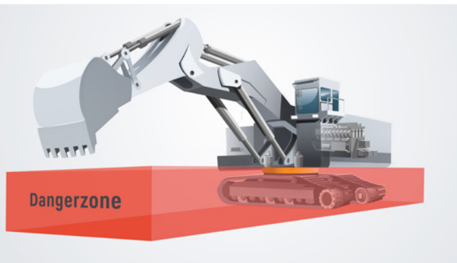
The danger zone of the excavator is located directly at the point, where the service personnel attaches the measuring device during manual measurement.
