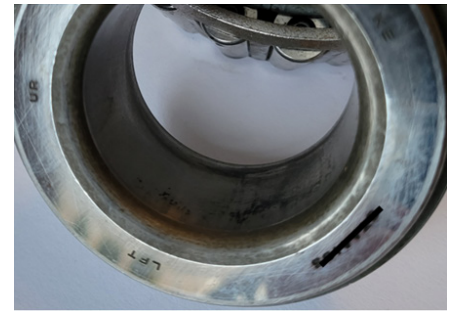
Tested Bearing: Mirror surface, reduced grind lines: Bearing has been turning
