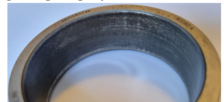
OBJECTIONABLE: Heavy thermal staining. Heavy wear lines.
