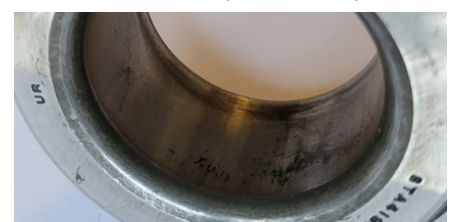
Light thermal marks at edges. Light indications of turning. No tactile damage. Possible pass.
