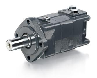
operating pressure, the balance plate relaxes, allowing the rotor to turn freely which translates into higher mechanical efficiencies. Transmitting this power to the output shaft is the most durable drive link in its class. Four bearing options, combined with standard mounting flanges and output shafts, allow the motor to be configured to suit nearly any application.
