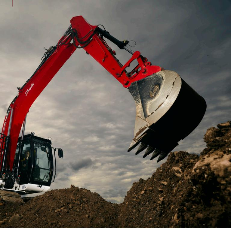
provides unique digital flow control, resulting in vastly improved system efficiency and faster operator response times. Through the fast response and digital control of the hydraulic pump, engine loading can be controlled, providing significantly reduced fuel consumption without compromising on productivity.
