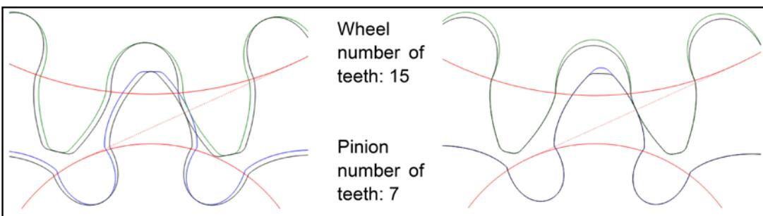
Figure 4 Left—complementary toothing; right—pinion addendum and wheel dedendum increased.
