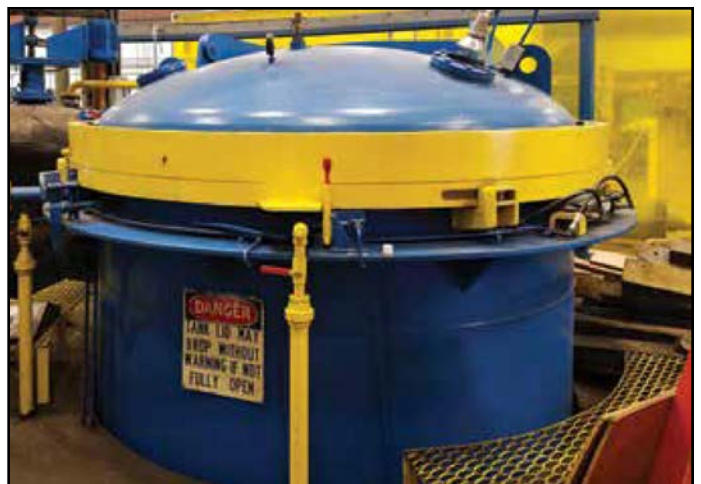
Figure 3 Eight-foot vacuum pressure impregnation (VPI) system at EECO’s Industrial Motor Services in Richmond, VA.
