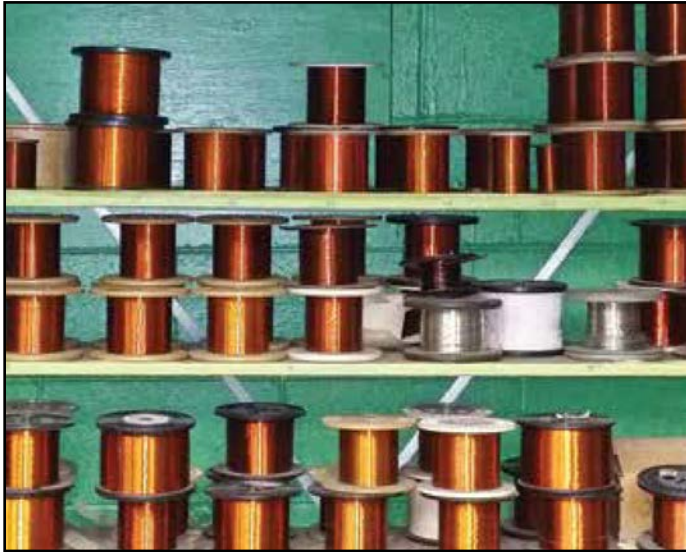
Figure 2 Rolls of new copper wire used in motor rewinds at FLOLO.
