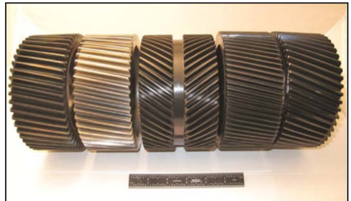
Figure 5 Photograph of input gear designs; baseline, baseline + ISF, double-helical, fine pitch, and increased helix angle.
