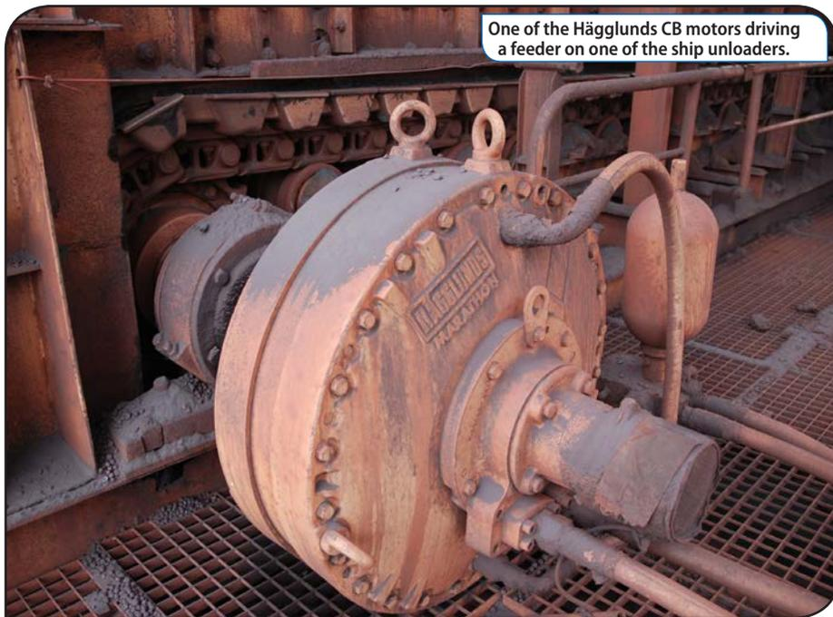
One of the Högglunds CB motors driving a feeder on one of the ship unloaders.
