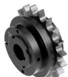
The EDF/F series is a ball torque limiter, which consists of two halves: a driving member and a driven member that are separated by a set of steel balls housed in grooves on both members.
