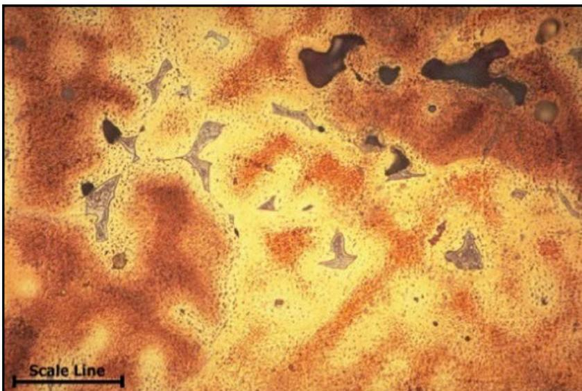
Figure 2 Microstructure of tin bronze as cast (scale line length ~50 microns) (Ref. 8).
