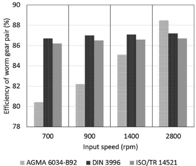
Figure 5 Efficiency of worm gear pair (gear ratio = 28, center distance = 150 mm) as a function of input speed based on the analytical calculation from AGMA, DIN and ISO standards.
