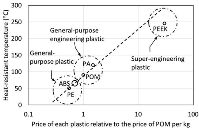
Figure 4 Heat-resistant temperature as a function of relative price to the price of POM per kg for plastics used for worm drives (Ref. 37).
