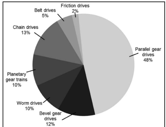
Figure 1 Global distribution of mechanical power drives in which worm drives make up approximately 10 percent of all drives (Ref. 1).
