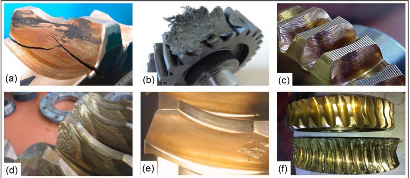
Figure 3 Wormgear failures: a) tooth breakage (Ref. 25); b) deformation and melting of plastic gear (Ref. 26); c) scuffing (Ref. 27); d) corrosion pitting (Ref. 28); e) pitting (Ref. 29), and f) wear — before (top gear) and after (bottom gear) usage.
