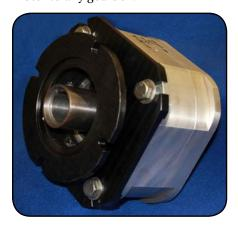
Consisting of a face mounted speed reducer with a hollow shaft input, these new designs function as gearheads. Built on the Nu-Lobe gear design, they are available in standard ratios of 3:1, 4:1 and 5:1, making them ideal for a wide range of industrial and commercial applications, including use on mixers, parking lot gates, wind turbine yaw drives, conveyors, hoists and other material handling equipment, food processing equipment, robotic drives and more.
