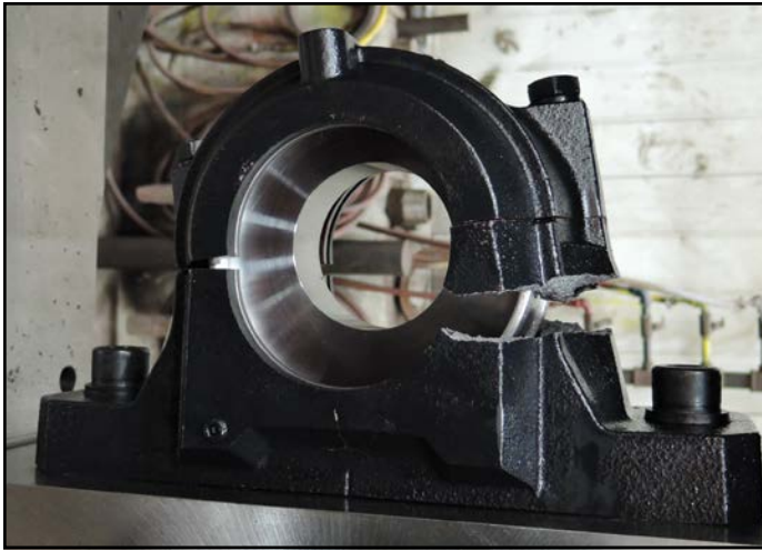
Figure 6 Fracture of split housings.
