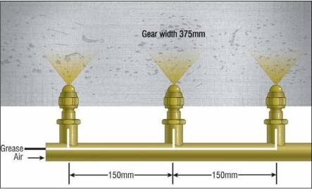
Figure 2—Placement of spray nozzles; example of three-nozzle spray bar with spray nozzle spaced apart at 150 mm.
