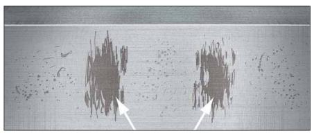
Figure 3—Inadequate spray pattern on the tooth flank; inadequate spray patterns normally lead to scuffing in these highlighted areas. Additional, correctly spaced spray nozzles and higher air pressure are required to improve the lubrication film.
