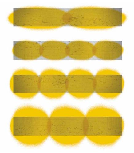
Figure 1—Correct lubricant spray patterns on tooth flanks.
