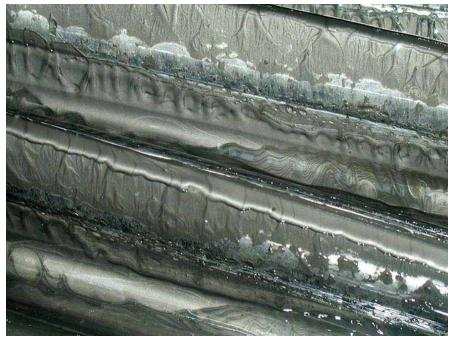
Figure 7—Over-lubricated open gear.
