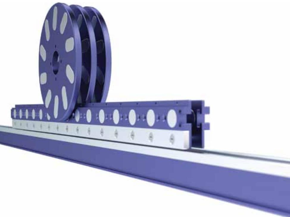
magnetic wheels can be used either as gears or couplers. If the system is overloaded, it simply slips, avoiding potentially dangerous situations. Coupler faces don't touch, so no vibrations are transmitted.
