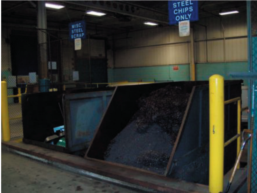
Separating miscellaneous steel scrap from chips is merely the first step in byproduct synergy where one company's waste is identified for reuse by another company. (Courtesy of Gleason Cutting Tools.)
