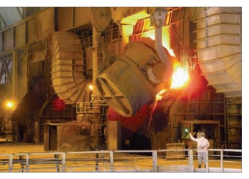
A WEG turnkey system including transformers, MV motors and MV frequency inverters is used to automate a crane that carries molten metal at a plant in Brazil. Usiminas, a producer of iron and steel, employs the crane, which is one of the very few in the world to be controlled by a PLC and digital frequency inverters connected over the Profibus-DP communication network.
