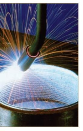
Bortech Corp. recently introduced BoreClad, a new system for weld overlaying and restorative buildup. The system is used for applications in restoring worn construction, industrial and military equipment, pit, quarry and mining processes and other parts needing rebuilding due to abrasive wear.
