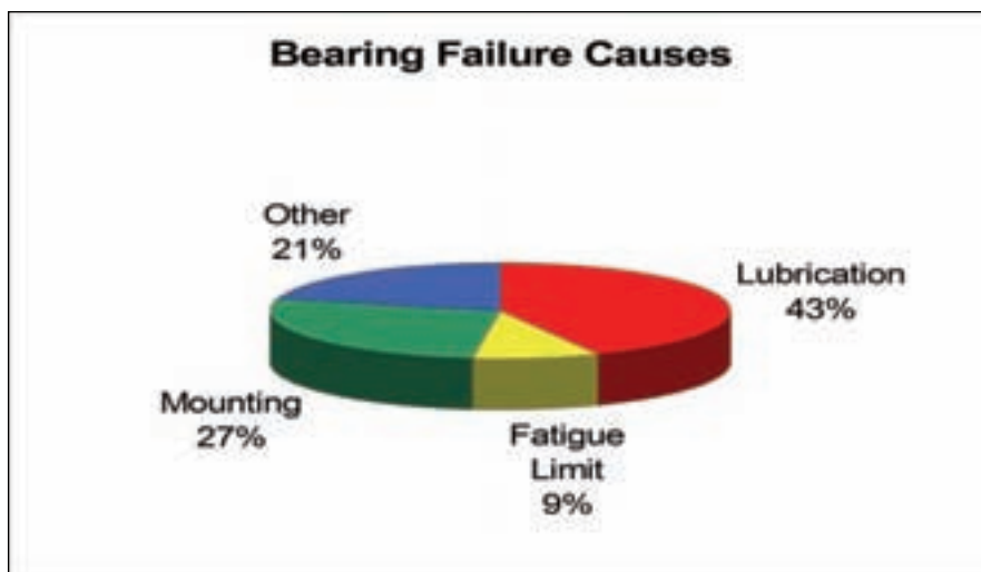
Figure 1—Degraded lubrication is the No. 1 cause of bearing failures.
