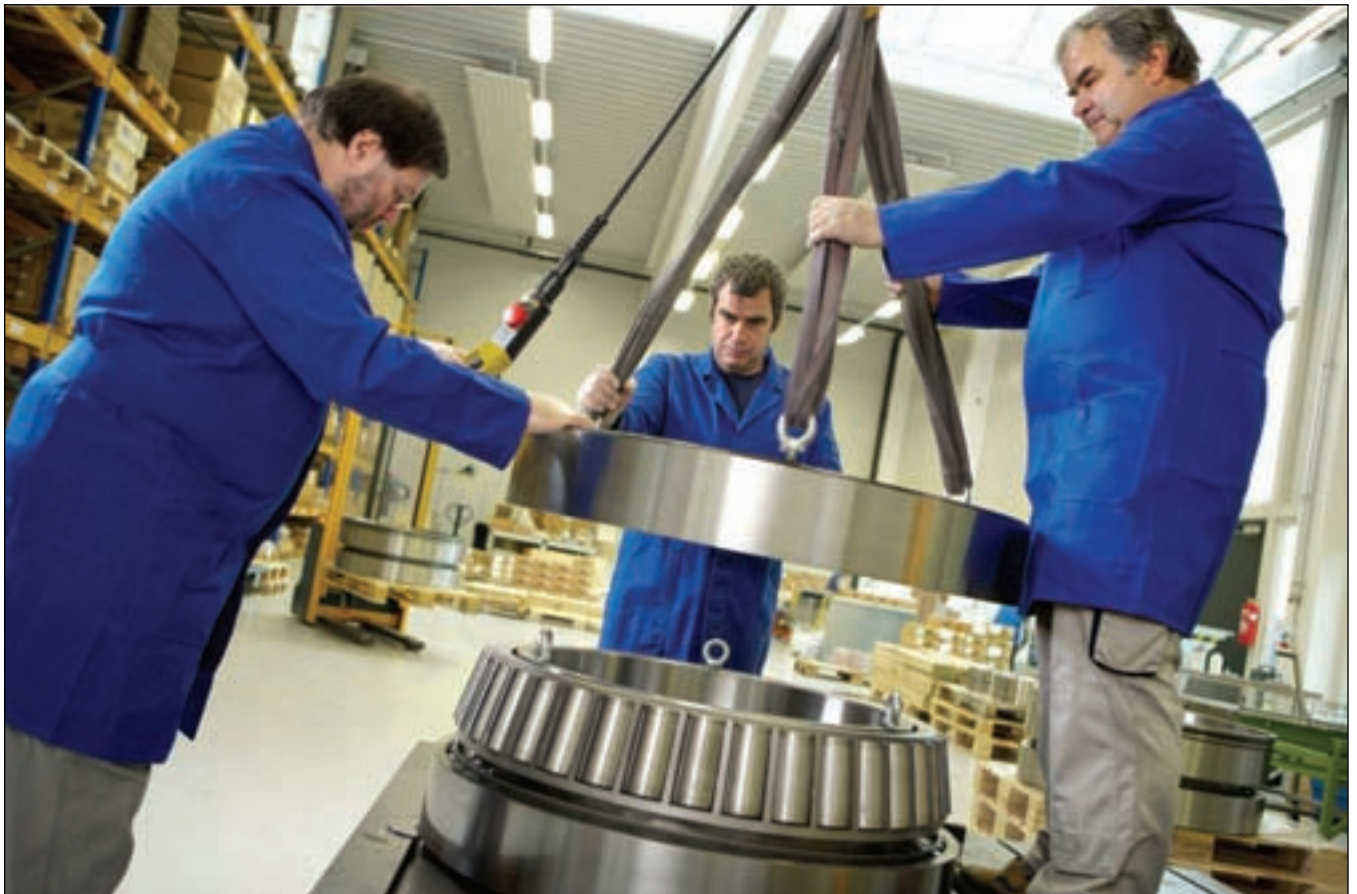
Only the highest-grade steel—typically sourced in Western Europe—is specified for wind turbine bearings. Here we see workers at NKE's Austrian plant doing final assembly.
