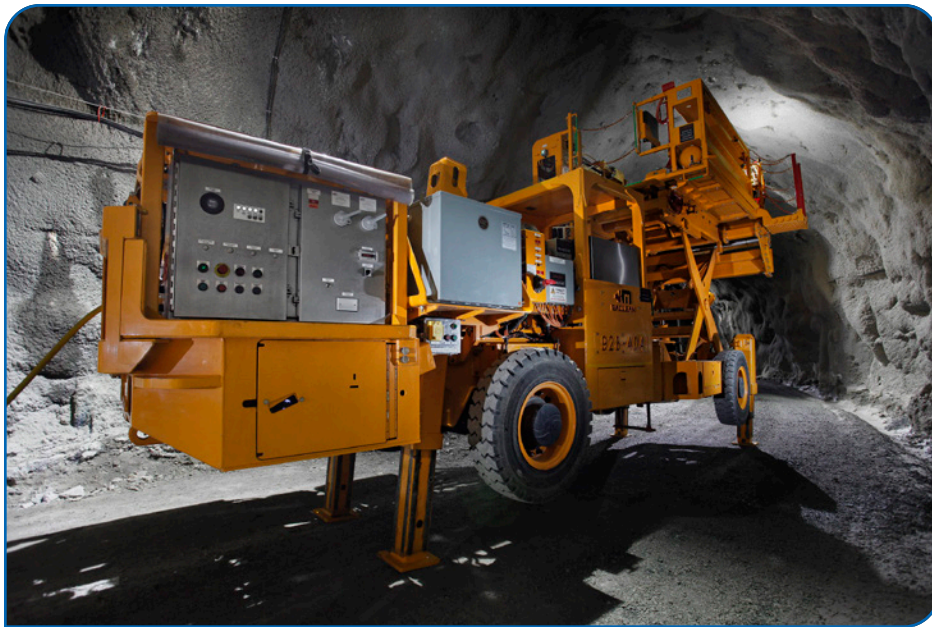
Maclean battery-operated equipment for underground mining.
