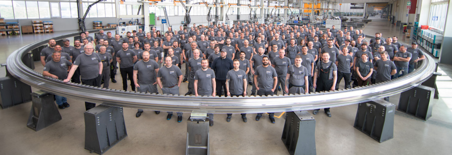
Liebherr's slewing bearing consists of 68 segments with a total diameter as large as six small cars in row. All photos courtesy of Liebherr.
