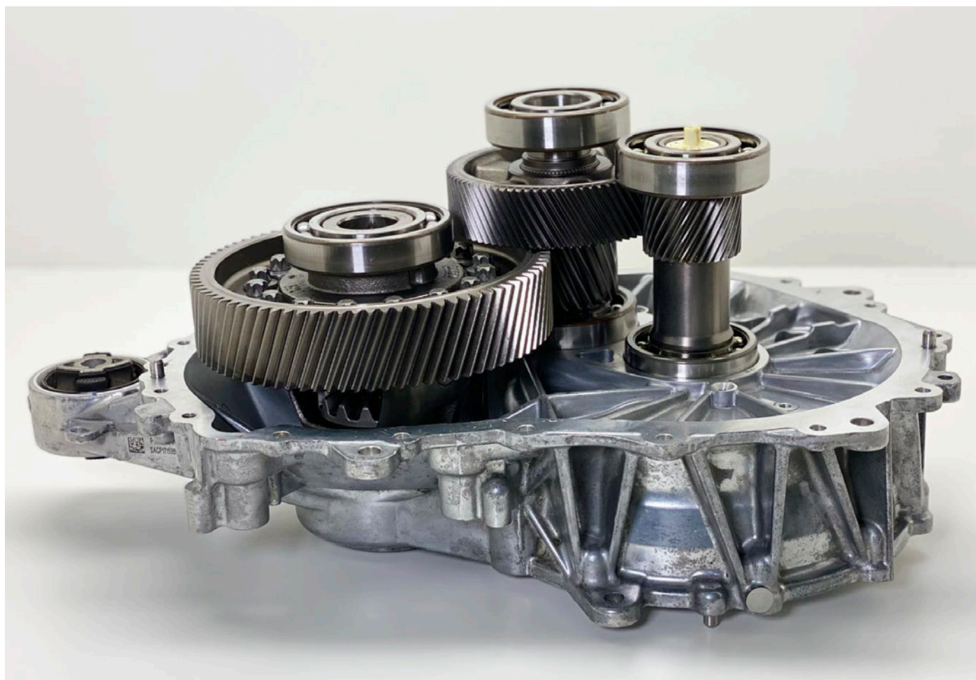
Figure 1—Photo courtesy of Munro Live on Instagram: "Partial Disassemble of the 2018 Tesla Model 3 Helical Gearbox." Instagram, 2017, www.instagram.com/p/COiQJ1rniM1
