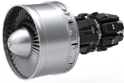
Capable of delivering up to 2.5 MW, the WM2500 motor has a power density of around 18-20 kW/kg.
